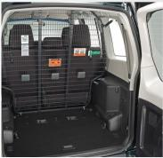
This practical accessory has been engineered to withstand the severe impact of a loss projectile that may be thrown forward in the event of strong braking or an accident. These loss is lems may in certain situations become missiles that can cause severe injury to occupants. Made from impact resistant steel, the Cargo Barrier has mounting points in 2 positions. It has been designed to provide a safe exit from the Cargo Area to avoid entrapment and includes an integrated class breaker.
