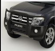
The Pajero's genuine Steef Front Protection Bar is made from pressed steel components. Lie all Missubsisting jenutine protection bars, it has been specifically made explorering standards and is alrivag compatible. This bar also complies with bar was provided to the protection. The penume Front Protection Bar has net this Standard by adding energy absorbing panels onto the top of the bar. This means improved safety for you and other road users.
