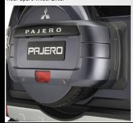
For towing with your Pajero, this unique accessory lifts the mounting point of the spare wheel mounted on the rear tailgate to provide additional clearance for towing equipment that requires additional height over the towbar.
