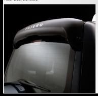
This stylish accessory is made from durable acrylic and mounts at the top of the tailgate. The Dust Deflector prevents the build up of dust and dirt that can collect on the rare window. It is especially useful for owners who live in the country and traverse dirt roads. It is also easily removed and reattached for cleaning. Note: Not compatible with Rear Reversing Mirror.
