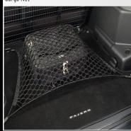
This accessory has been designed specifically to prevent loose items in the rear of the Pajero from moving around. The net clips to existing anchorage points in the cargo area of your Pajero.
