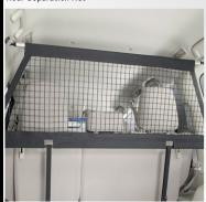
Not suitable for 2WD Pajeros, this accessory separates the rear cargo space from the passenger area. Note: Only suitable to be fitted behind
