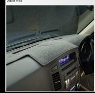
The genuine dash mat is designed to suit the contours of the Pajero's instrument panel and also protects it from the harsh effects of the sun. It is made from carpet and features a moulded backing to allow for a perfectly integrated fit.
