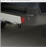
This is a very useful feature when reversing. A series of audible beeps indicates how close the vehicle is to an object, helping you judge the distance of your Pajero to obstacles when reversing or parking, it is available to match the vehicle colour and the sensors integrate perfectly with the Pajero's rear bumper.
