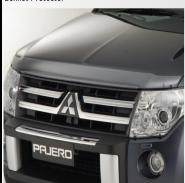
This Clip on Bonnet Protector is constructed of heavy duty aryclic and deflects flying stones from damaging the bonnet.
