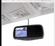
This Interior Rear View Mirror incorporates a built-in visual display screen that displays video signal from a camera mounted on the tailgate when reversing. Both camera and mirror are supplied.
