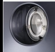
Designed specifically for the Pajero, these clip-on Foglamp protectors are made from heavy-duty acrylic to deflect flying stones neavy-outy acrylic to deflect riying stones from damaging your Pajero's fog lamps. They are easily removed and reattached for cleaning.Note: Sold as a set of 2 to suit left and right foglamps.
